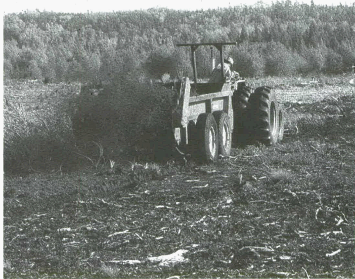
Equipment used to spread Sphagnum spores to accelerate restoration of a harvested peatland.
